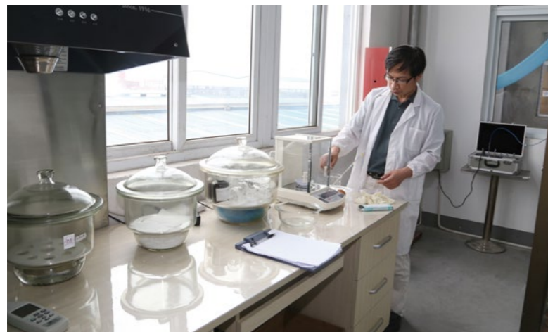
▲ CTC test system can test the Cl4 absorption performance for the activated carbon. It helps us evaluate the activated carbon quality.
