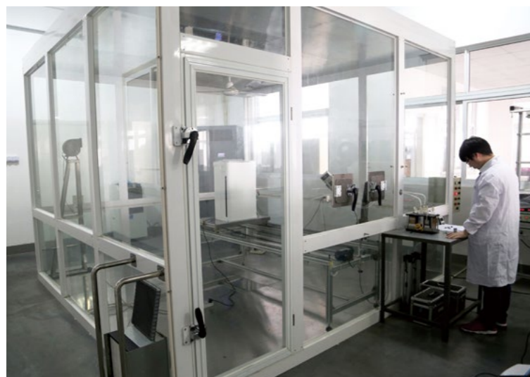
▲ 30m 3 test room for formaldehyde&VOC removing efficiency
