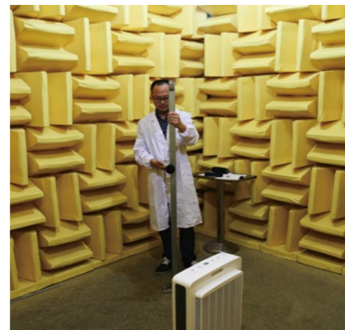
▲ Noise test lab can help us to evaluate the noise data for the unit.
